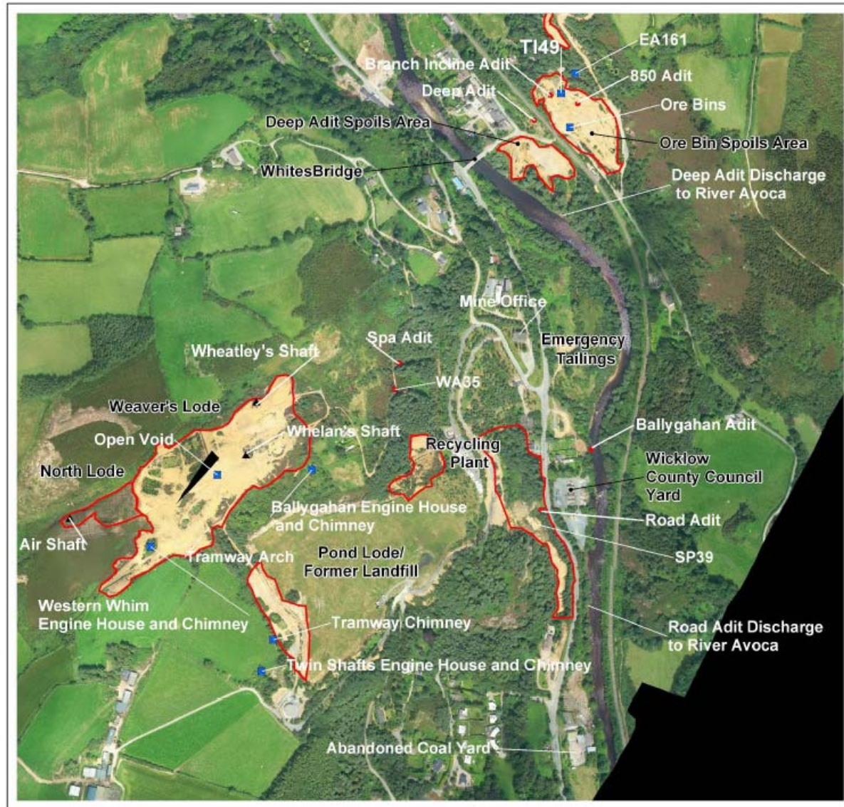
Figure 5-2: Location of spoil heaps in West Avoca (From CDM, 2008)
