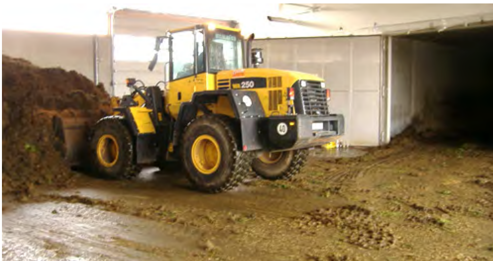
Fig. 3. Filling of a fermentation chamber with Bio-waste.
