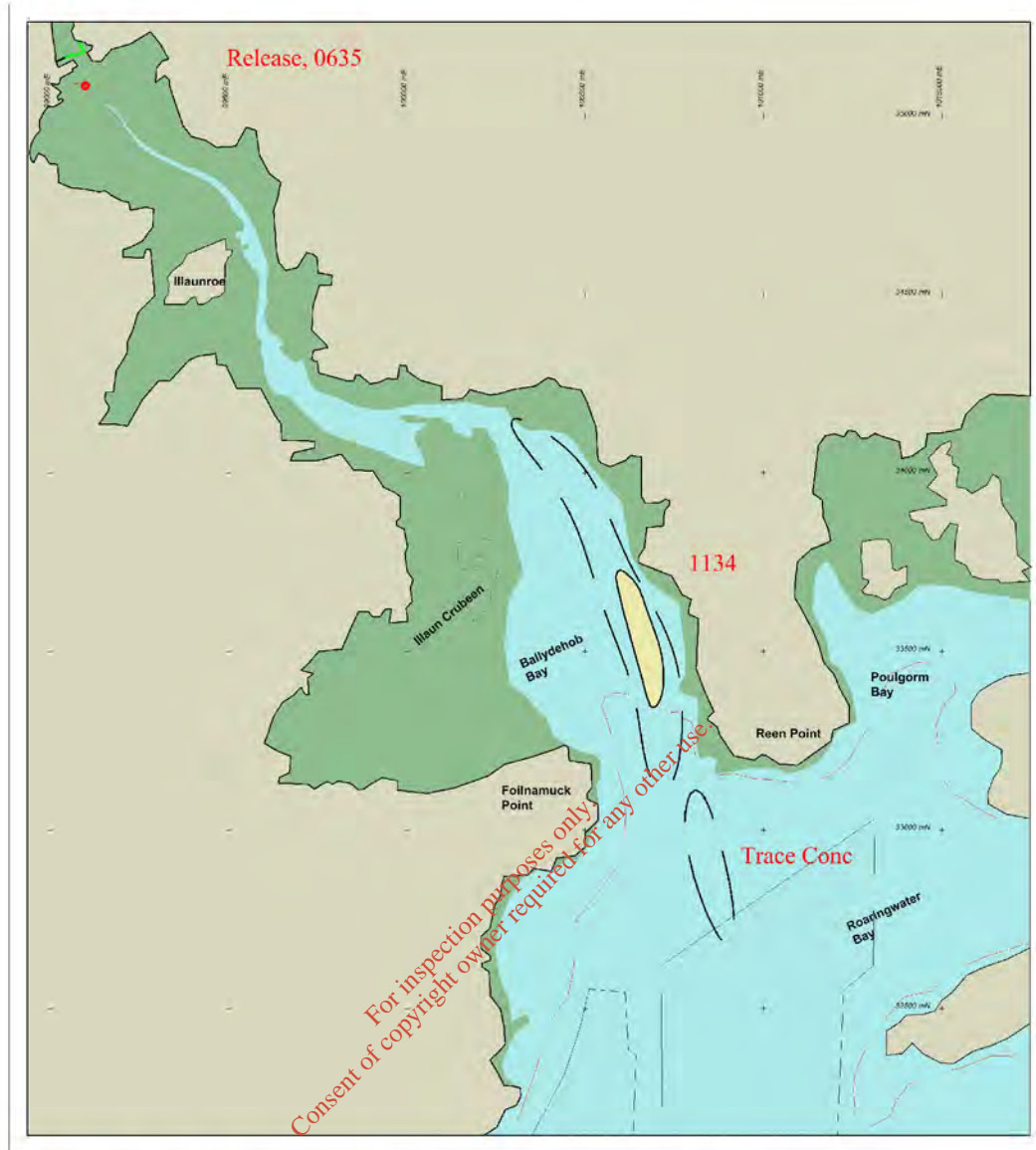
Figure 2.7b – Spring Tide Dye Release (contd), patch position at 1134hrs.
