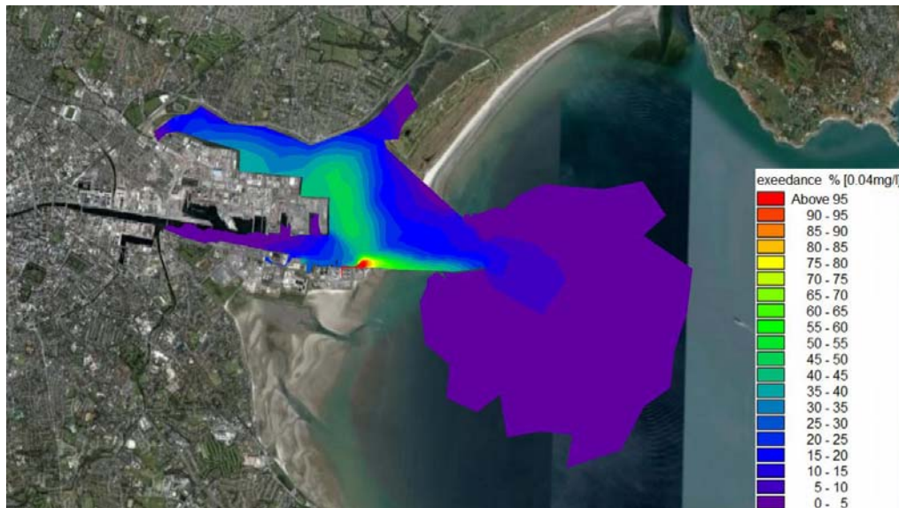
Figure 15: Exceedance values for concentrations larger than 0.04mg/l P for Scenario 5, Extreme Storm Event without wind.
