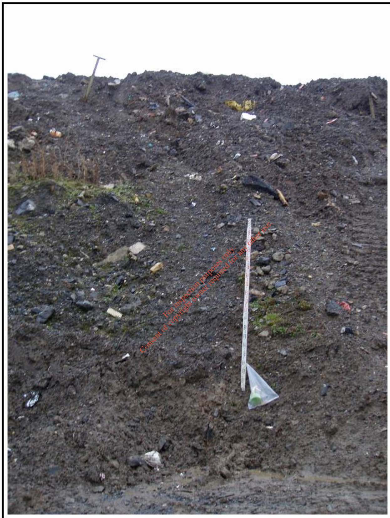
Plate A17: Profile of consolidated subsoil at the western edge of the main (western) fill area. This material is relatively clean throughout.
