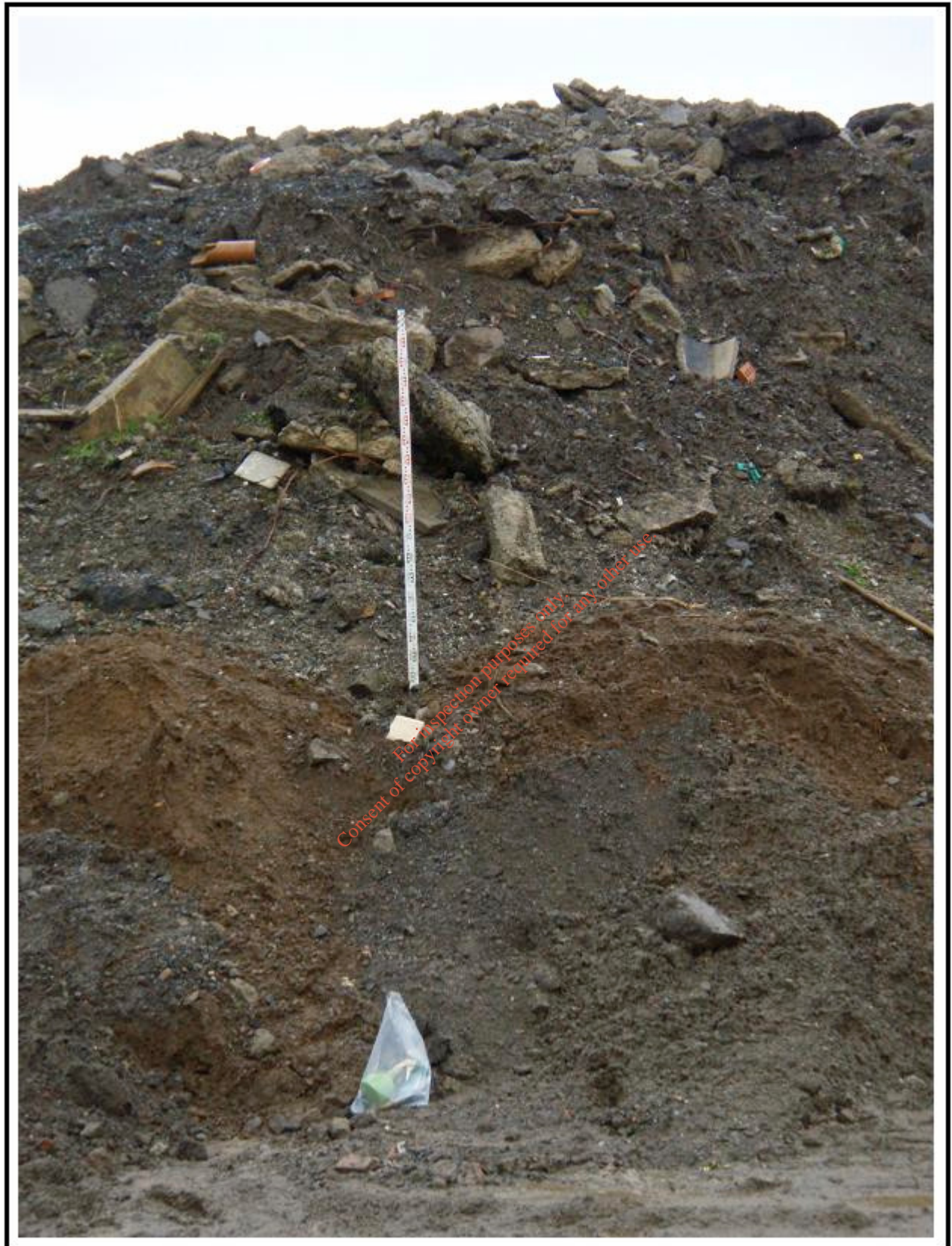
Plate A11: Profile of skim of recently-lain topsoil overlying consolidated subsoil at the northwestern corner of the main (western) fill area. Though containing much concrete at the face, this material is very clean throughout.
