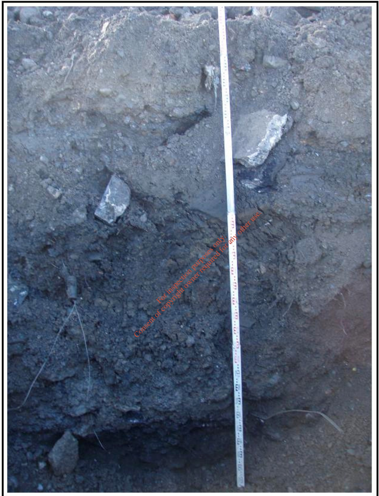
Plate A5: Profile of recently-filled subsoil in trial hole no. 5. Pieces of concrete and boulders are common in this area of the site also, with alternating compacted layers and occasional construction and demolition material.
