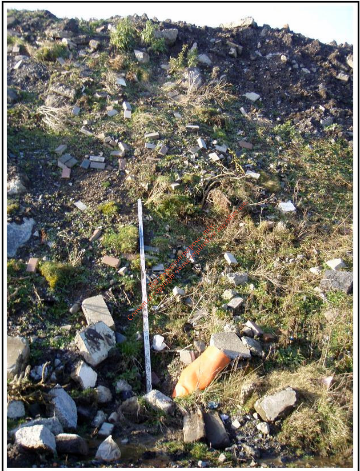
Plate A16: Profile of consolidated subsoil at the northeastern edge of the main (western) fill area. This material is also relatively clean throughout.
