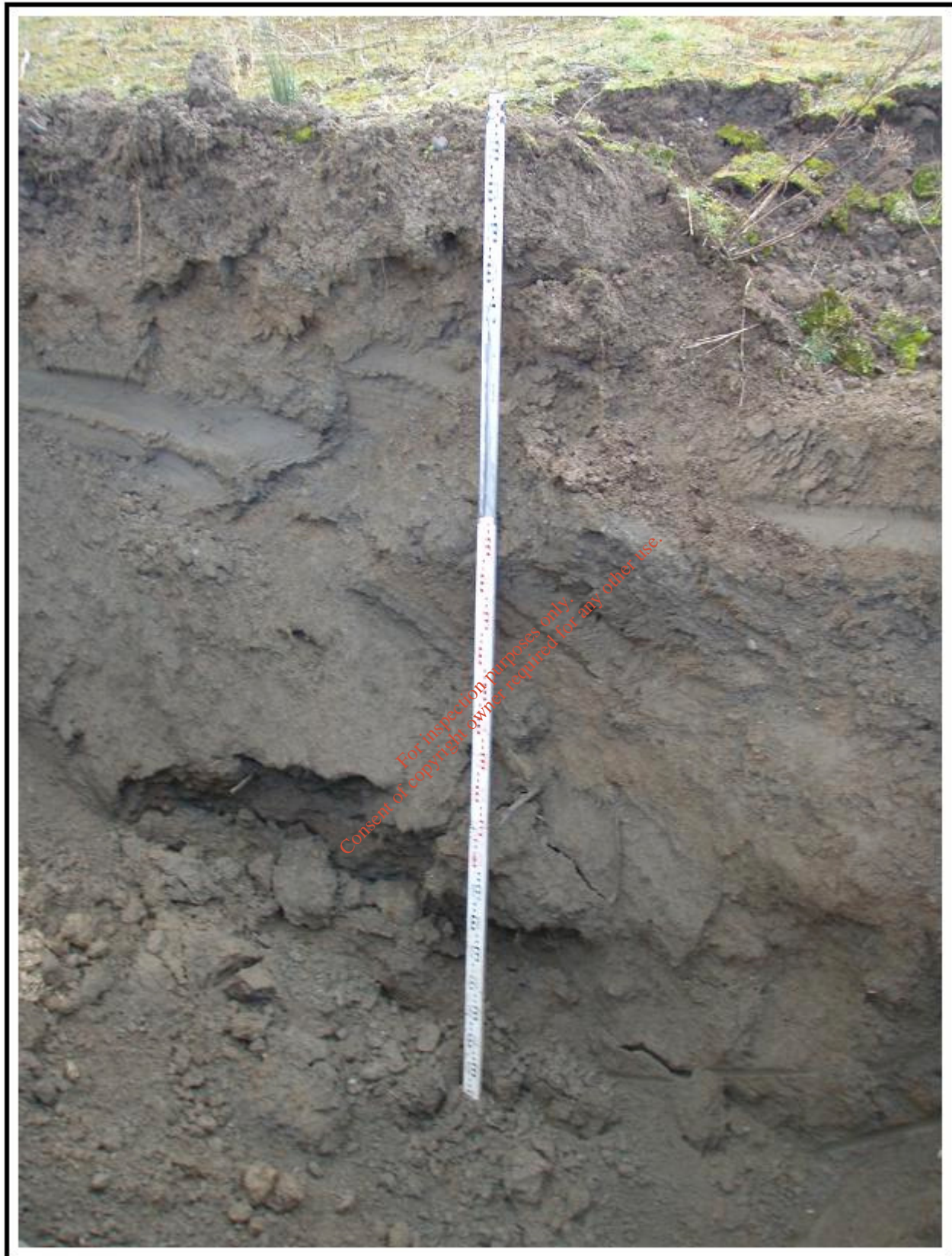
Plate A3: Profile of imported silty SAND topsoil and subsoil in trial hole no. 3. This is well drained topsoil taken from the adjacent gravel pit, with virtually no construction and demolition material within.
