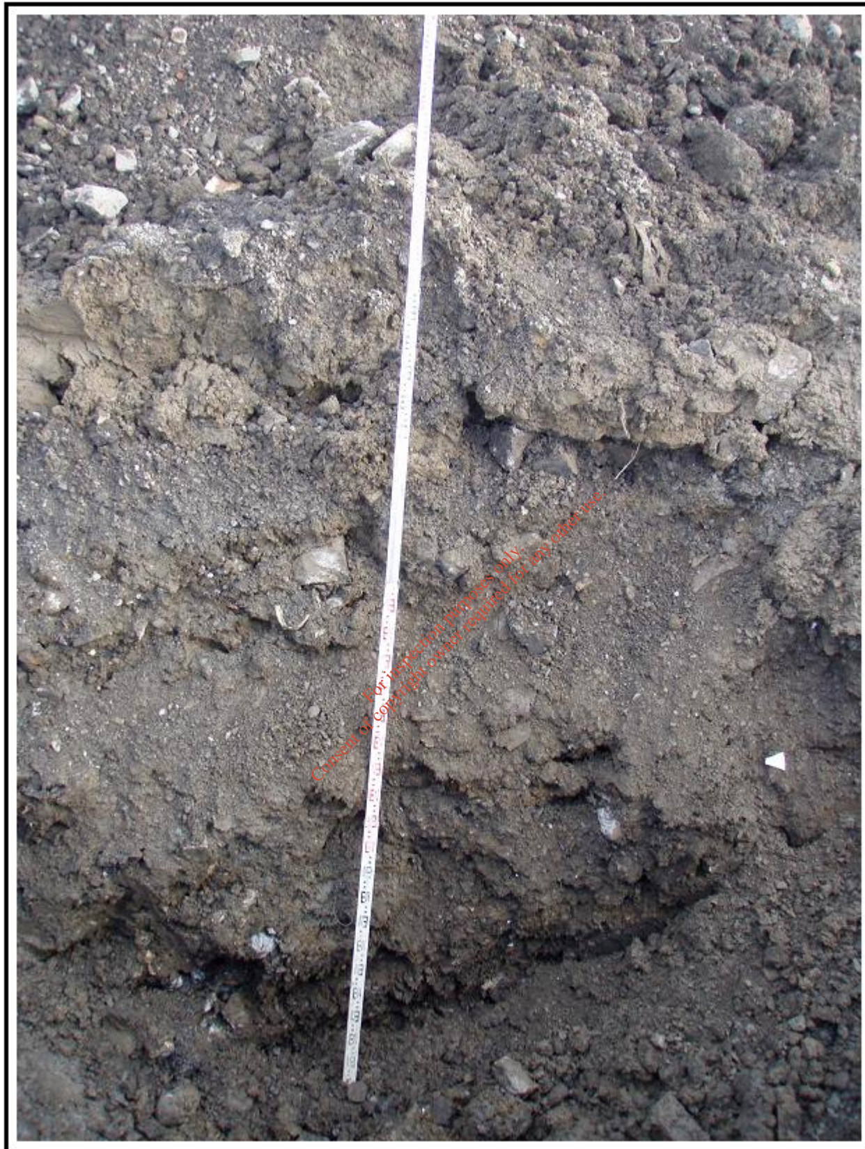
Plate A9: Profile of recently-filled subsoil in trial hole no. 9. Occasional pieces of concrete, branches and steel are seen, within alternating layers of compacted subsoil.
