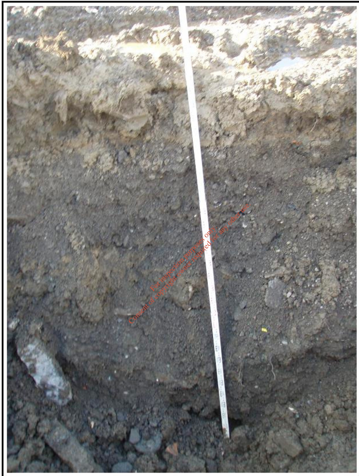
Plate A10: Profile of recently-filled subsoil in trial hole no. 10. This exposure shows little construction and demolition material, within alternating layers of compacted subsoil.
