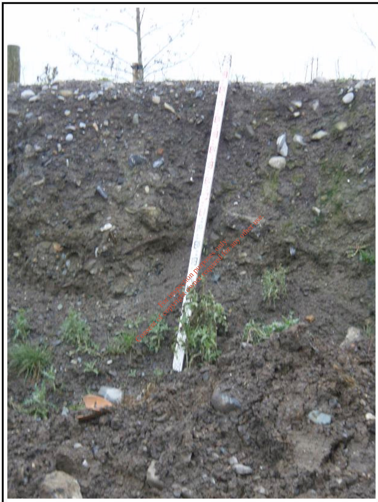
Plate A16: Profile of relatively shallow exposure into subsoil at the eastern extreme of the fill area. This material is also very clean.
