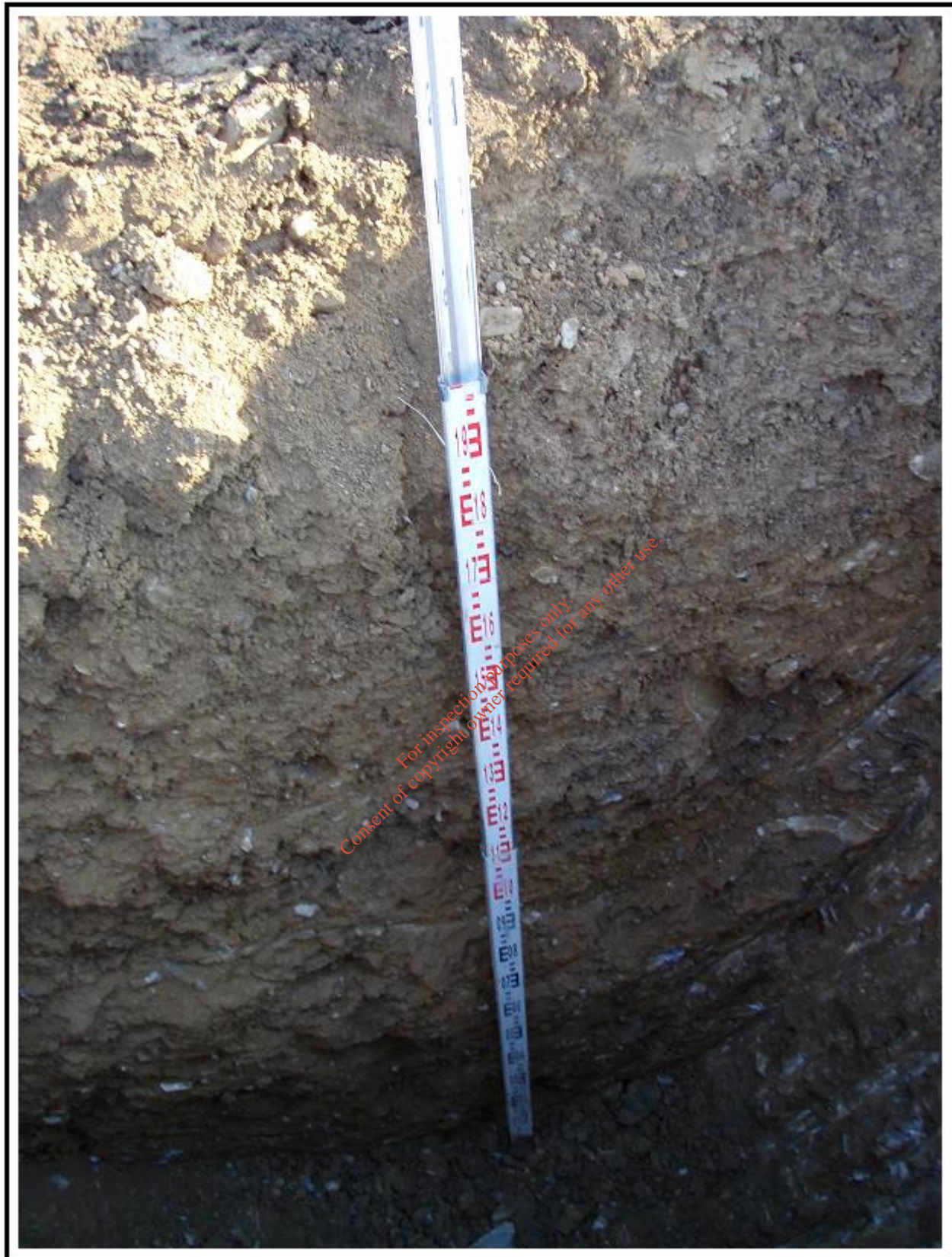
Plate A10: Profile of relatively shallow topsoil overlying overconsolidated, very stiff to hard subsoil in trial hole no. 10. See again the complete absence of waste material in this in situ subsoil material. The topsoil is of slightly better quality here and the subsoil is slightly more aerated. The hole was dry to 2.25m depth.
