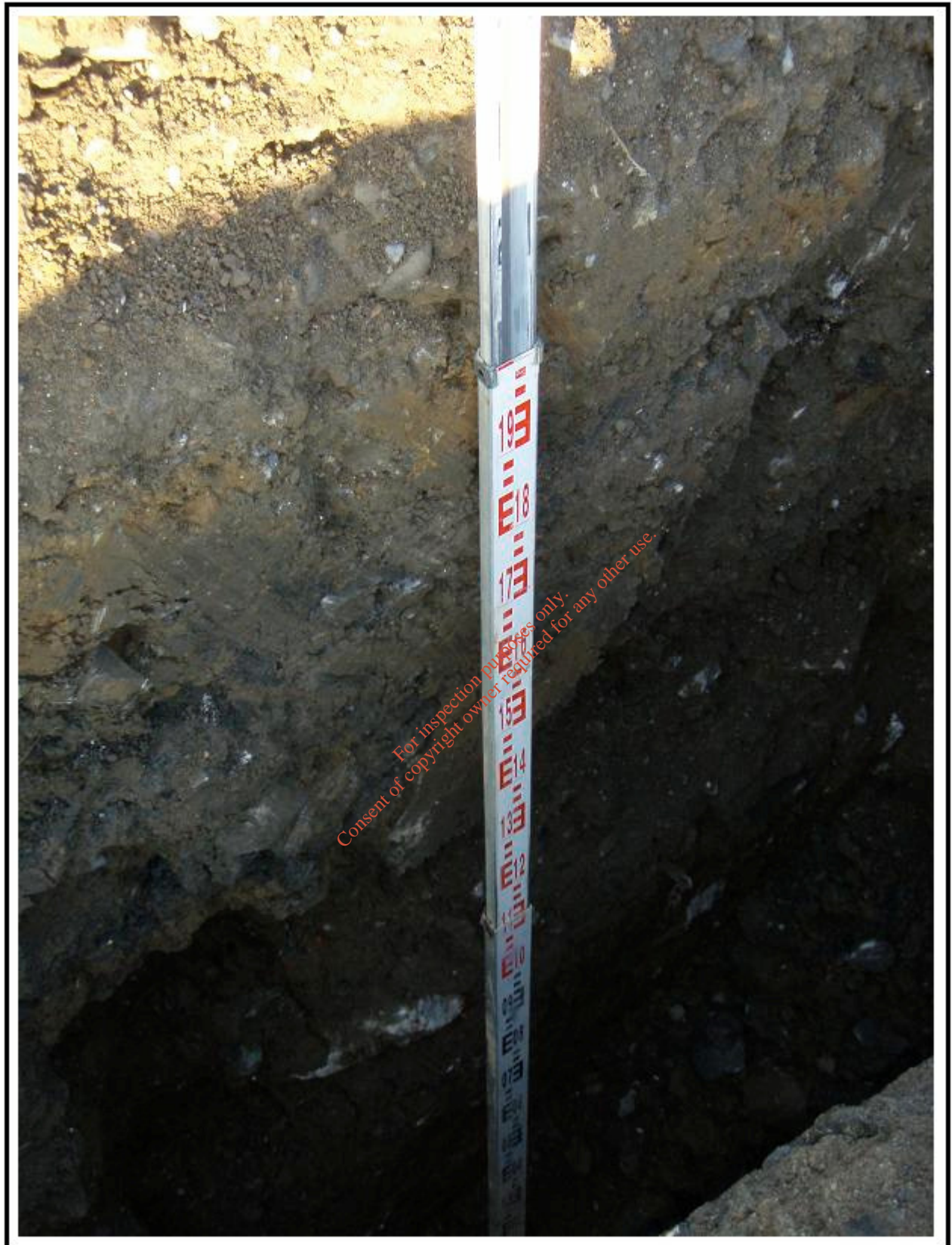
Plate A12: Profile of overconsolidated subsoil with alternating layers of very soft to stiff material in trial hole no. 12. Here also some buried pieces of concrete are seen at depth. No topsoil has been emplaced above this material as of yet, and the ground is bare.
