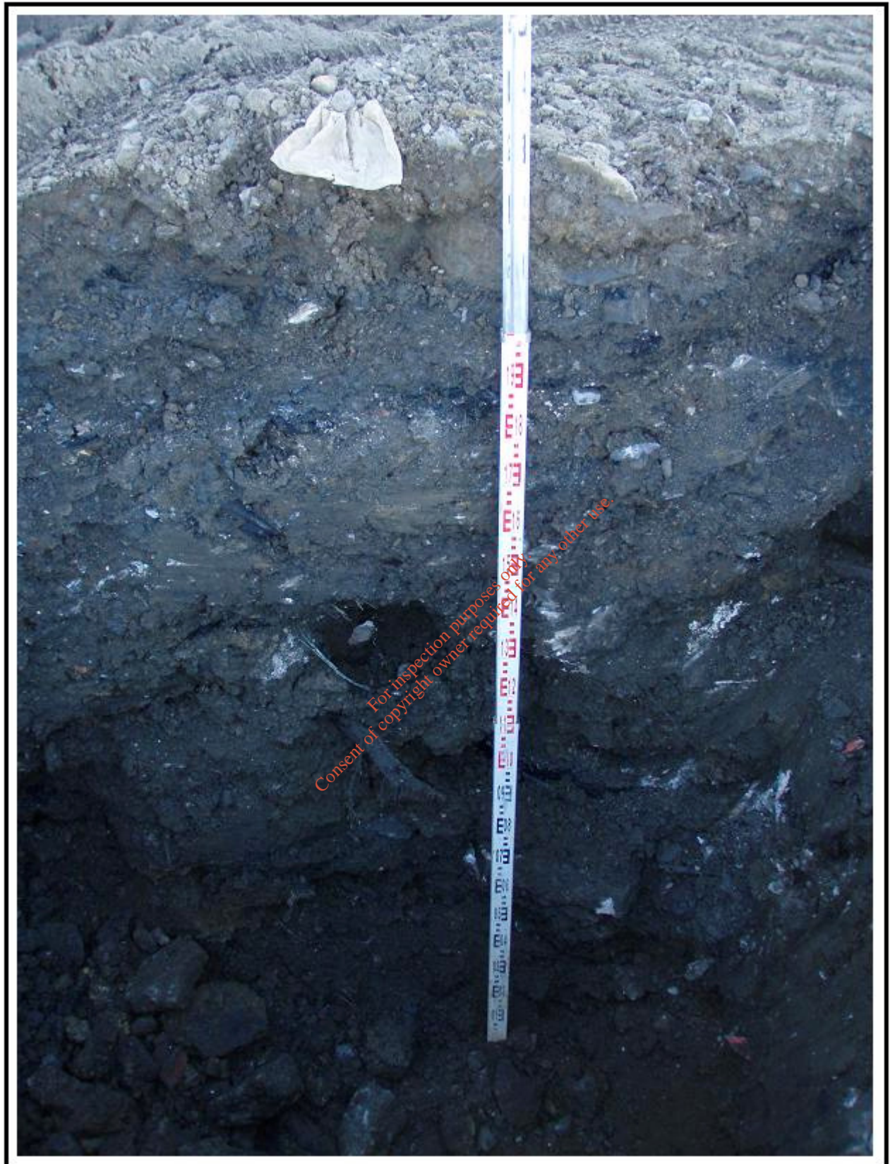
Plate A13: Profile of overconsolidated subsoil with alternating layers of very soft to stiff material in trial hole no. 13. Buried pieces of concrete, wire, branches and cloth also occur. No topsoil has been emplaced above this material as of yet either, and the ground is bare.
