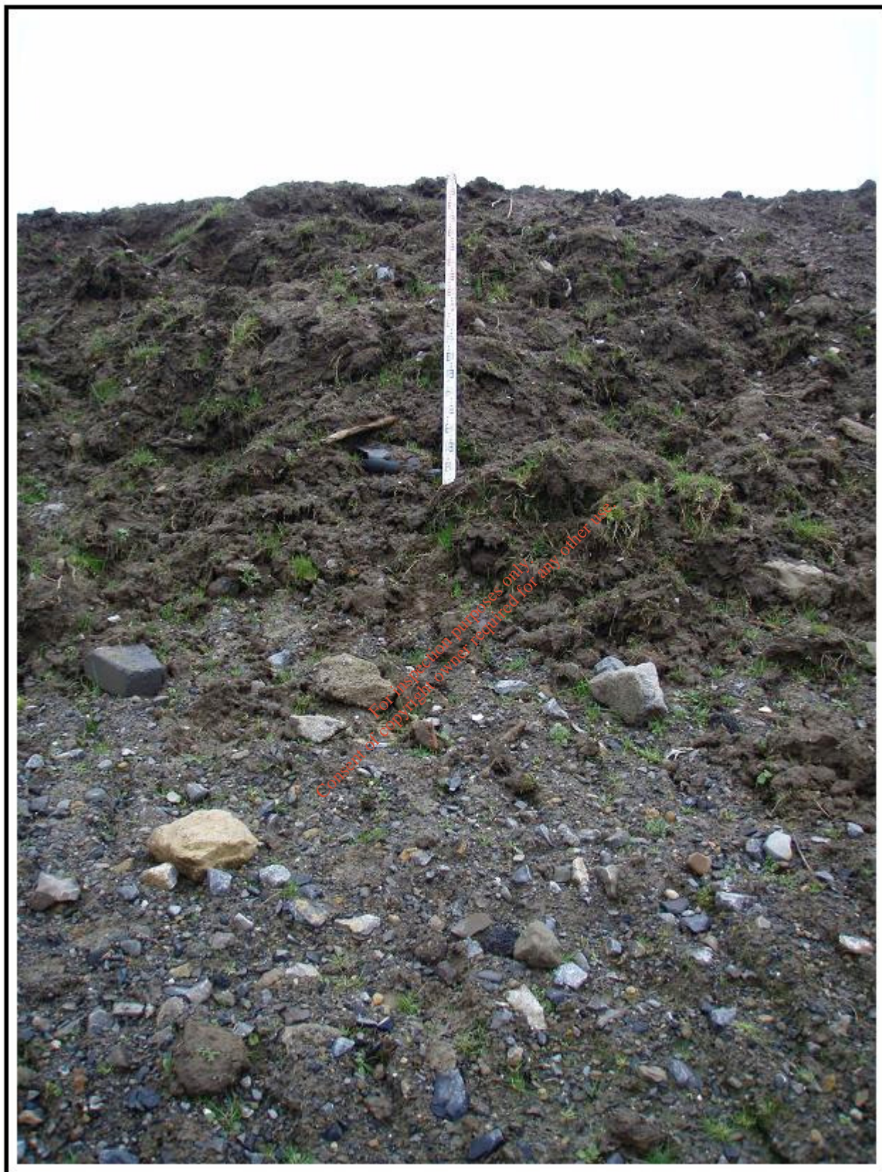
Plate A14: Profile of recently-lain topsoil overlying overconsolidated subsoil at the side of the main eastern fill area. This material is very clean with only one small portion of waste material (plastic pipe) seen.
