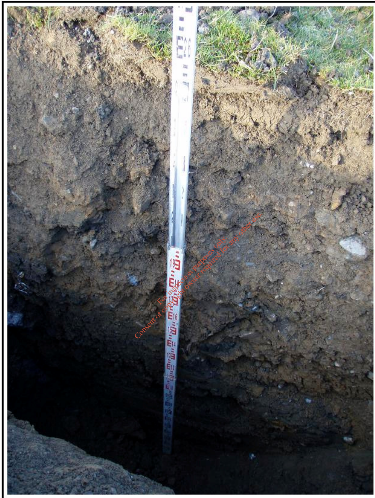
Plate A5: Profile of shallow topsoil overlying subsoil in trial hole no. 5. See the occasional concrete pieces and fragments of steel within the profile and the well aerated nature of the material, with no groundwater seepages recorded to 2.47m depth.
