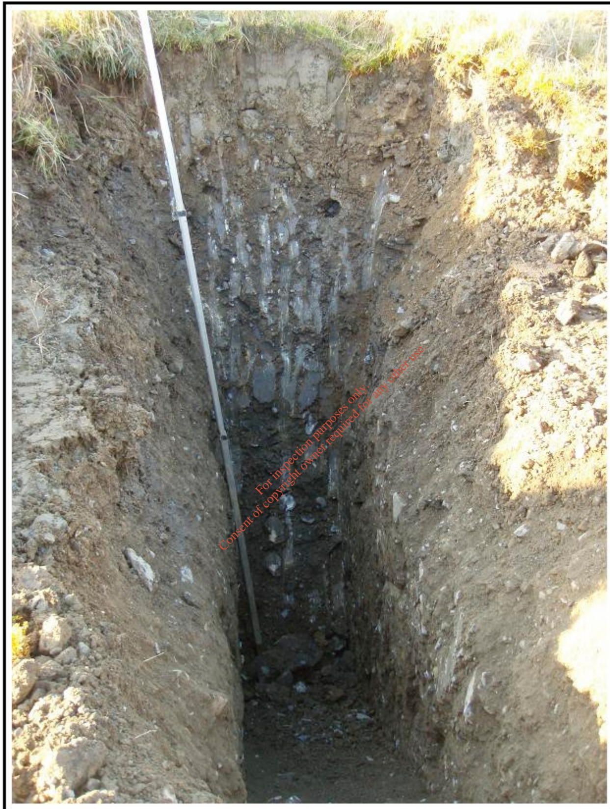
Plate A6: Profile of shallow topsoil overlying subsoil in trial hole no. 6. Surprisingly, given the low elevation, this hole was dry. See the complete absence of waste material in the clean in situ subsoil, with no groundwater seepages recorded to 2.8m depth.
