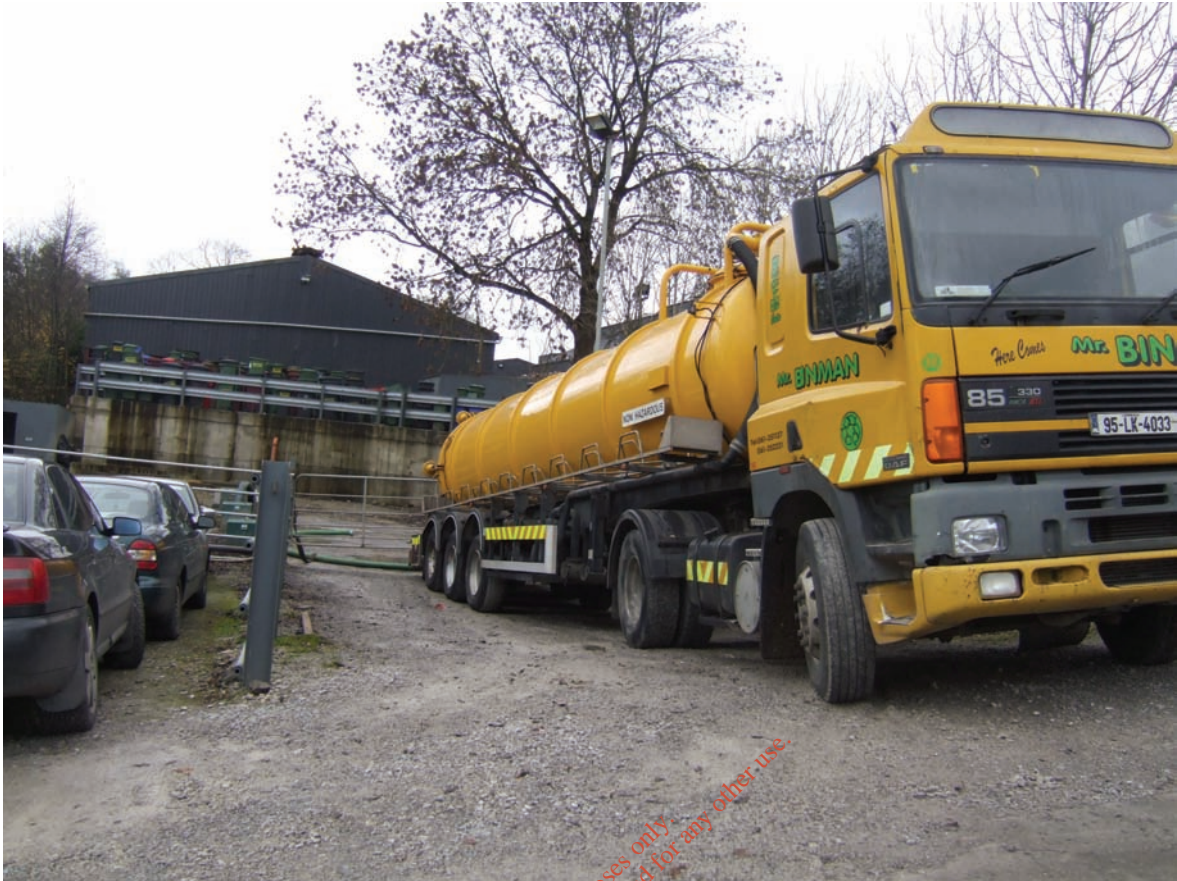
Plate 3.11 Treated wastewater is collected from the on-site treatment plant by truck
