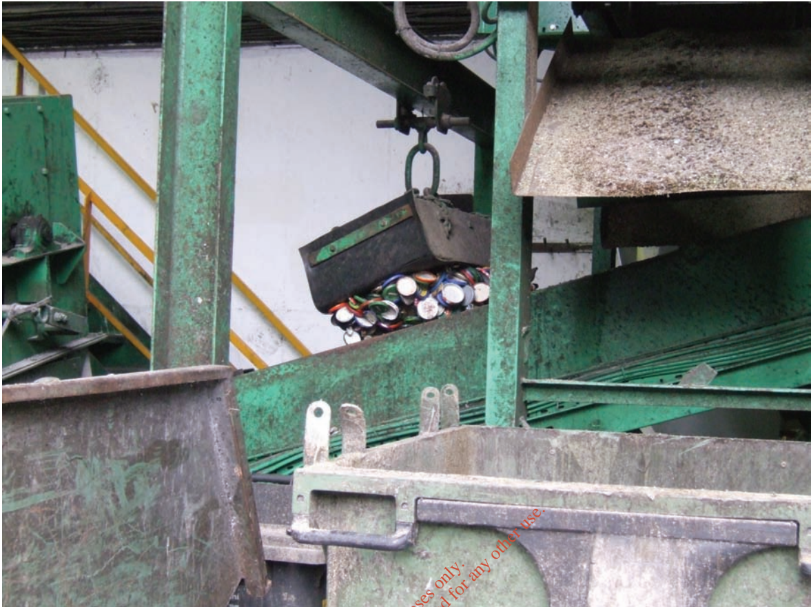
Plate 3.4 Removal of metal contaminants from waste glass stream by magnet
