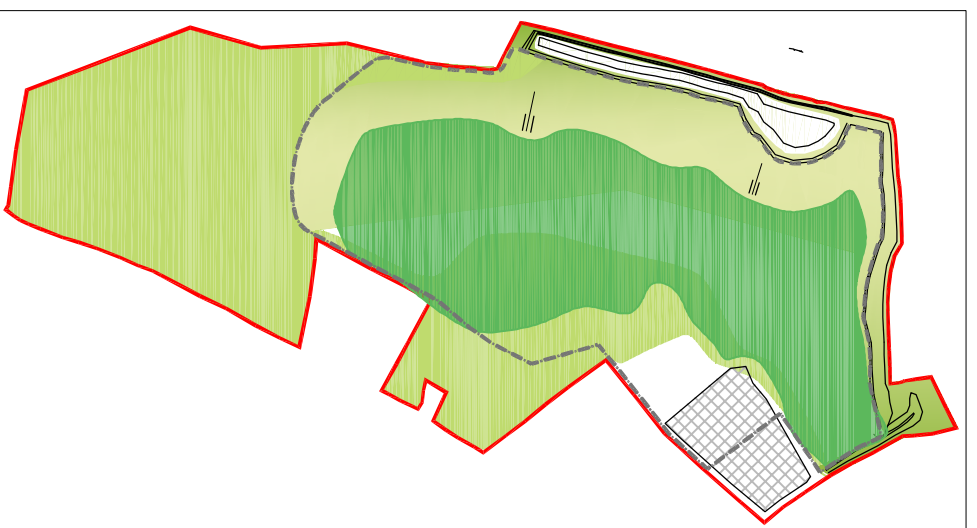
YEAR 6.0-8.5 INERT FILL FROM 154mOD TO 157mOD
