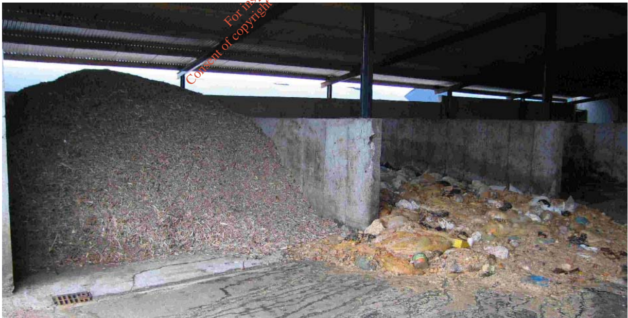
Separate feedstock storage bunkers at an on-farm in-vessel composting facility in County Carlow showing wood chips in one bunker to the left and commercial food in the bunker to the right.
