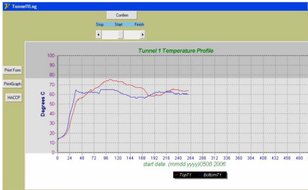
Typical time temperature graph from a tunnel composting facility in County Carlow illustrating the tracking of the temperatures in the top and bottom of the compost pile.
