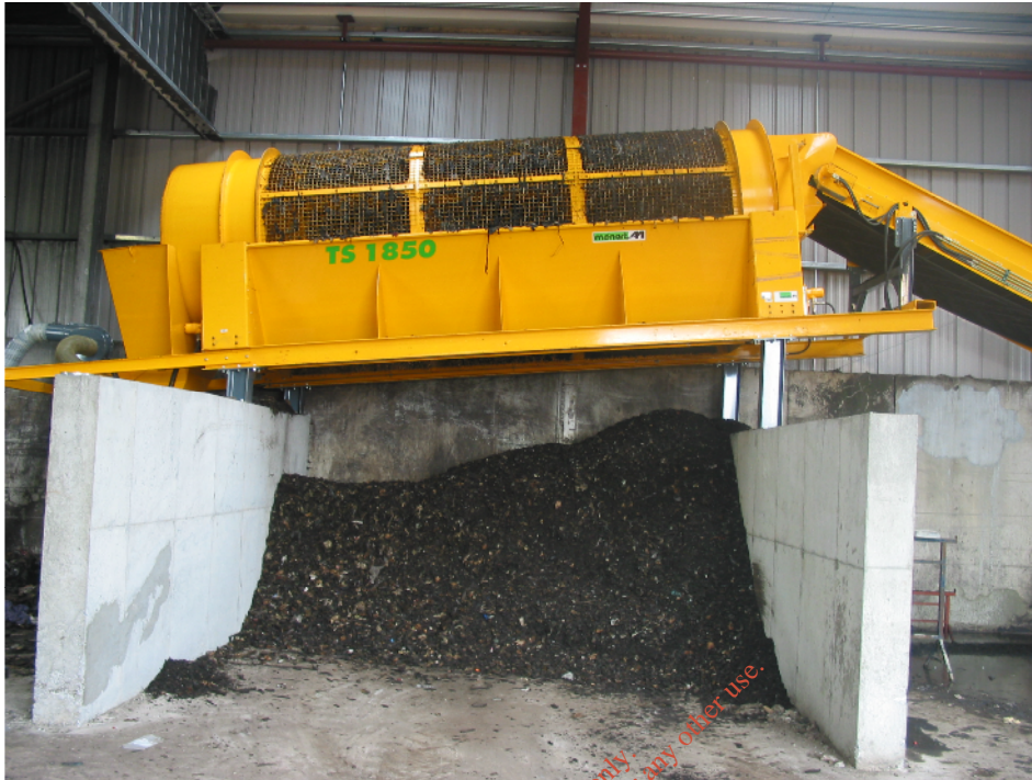
Stationary electrically powered trommel screen above from Galway City and star screen with air classifier shown below.
