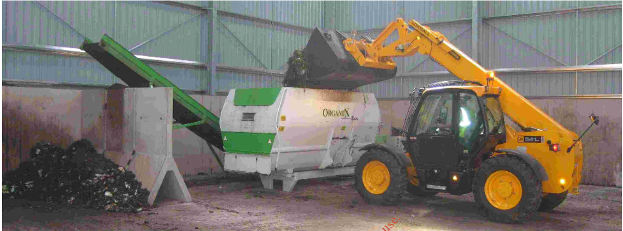
Loading stationary electrically powered batch auger mixer with biowaste for feedstock blending purposes.
