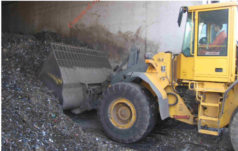
Front-end loader removing material from concrete tunnel
