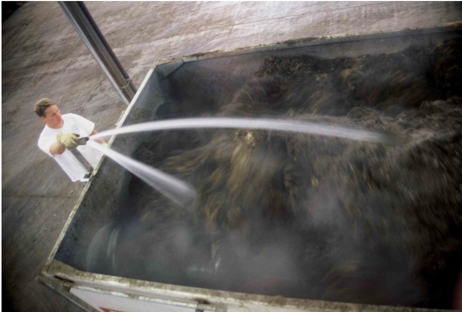
Water being added to a batch of feedstocks in an auger mixer at the end of the feedstock blending process.
