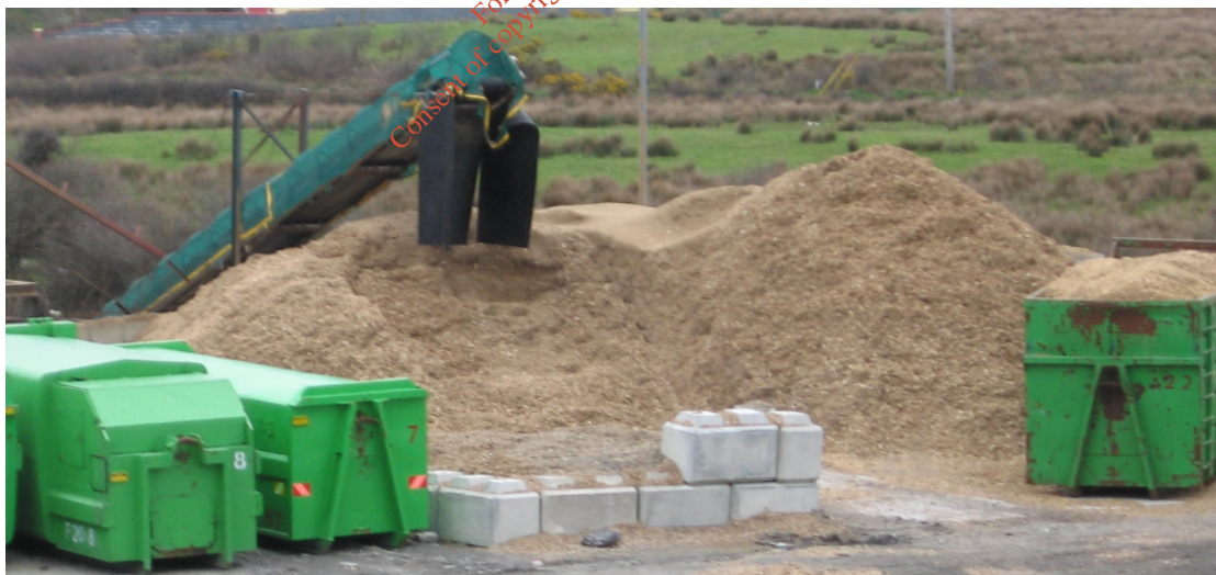
Top: Typical high speed shredder converting clean timber into wood chips. Above: Clean wood shredding area at CIRL site showing stockpile of processed wood chips. (Please note that a part of this overall planning and licensing application involves placing this whole shredding operation under roof.)
