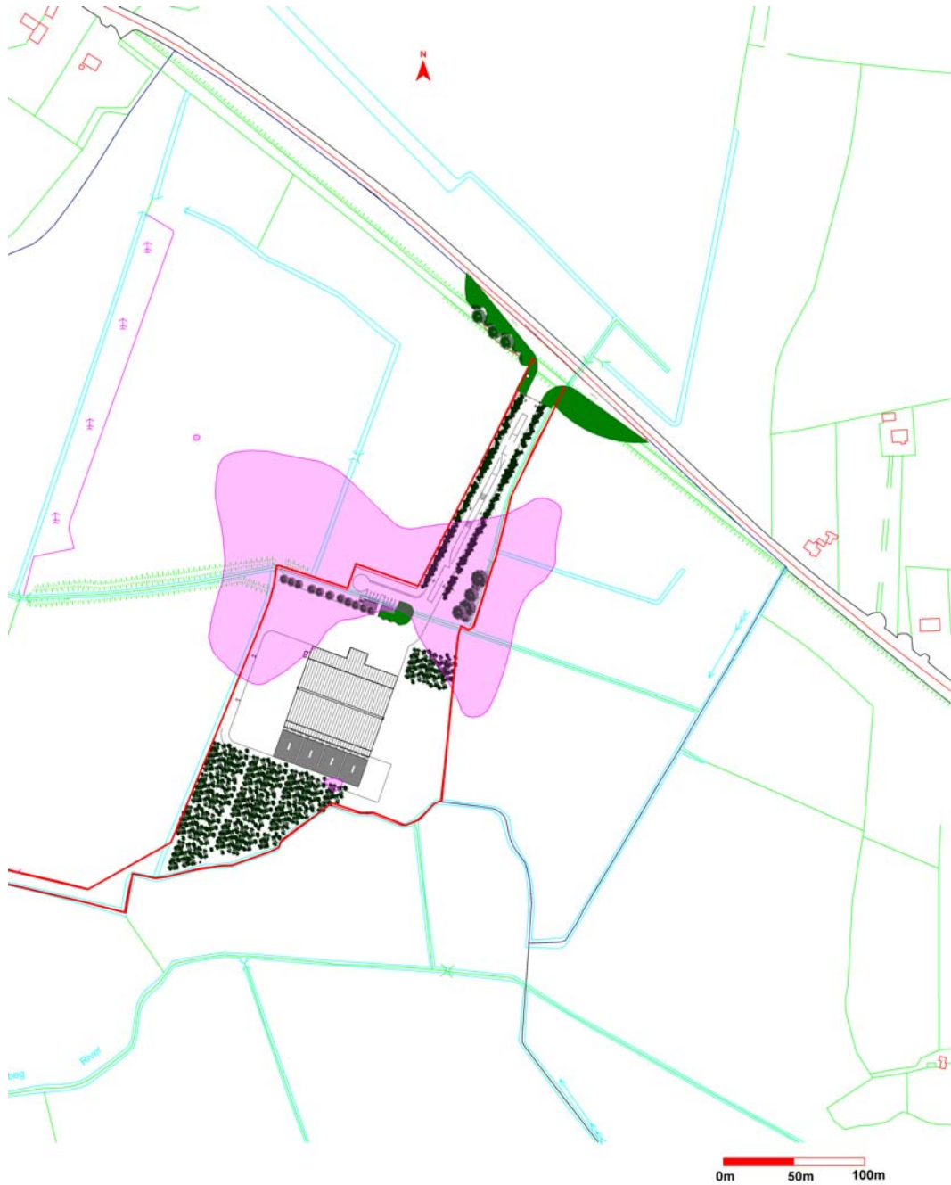
Figure 9.5. Predicted Total fungi emission contribution of proposed Littleton Recycling Facility operation to Total fungi plume dispersal for the 1 hour Total fungi plume spread for an Total fungi concentration of \leq 75 \text{ CFU m}^{-3} (—) for 7 years of hourly sequential meteorological data from Dublin airport (2000 to 2006 inclusive).
