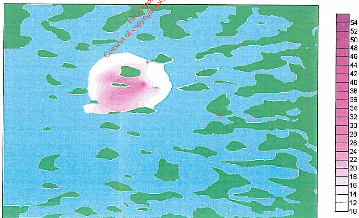
Figure A.33 : Copper concentrations (ng/l) at low water on a neap tide
