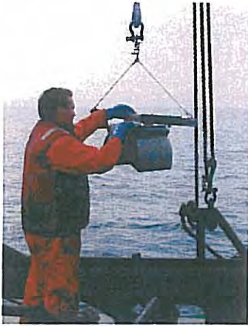
Plate 12.1. Van Veen grab used for sublittoral sampling.
