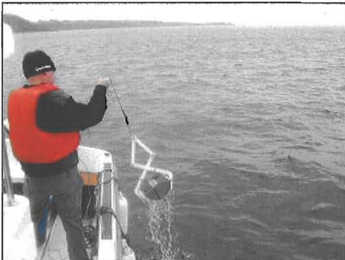
Plate B1 Grab sampling from a boat near the existing IDA outfall pipeline.
