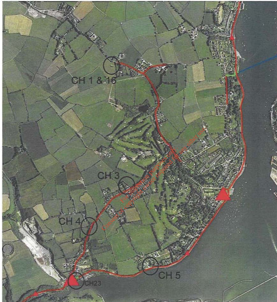
FIGURE 3.8.10 AERIAL PHOTO SHOWING CH LOCATIONS ALONG PIPELINE ROUTES IN THE MONKSTOWN AREA
