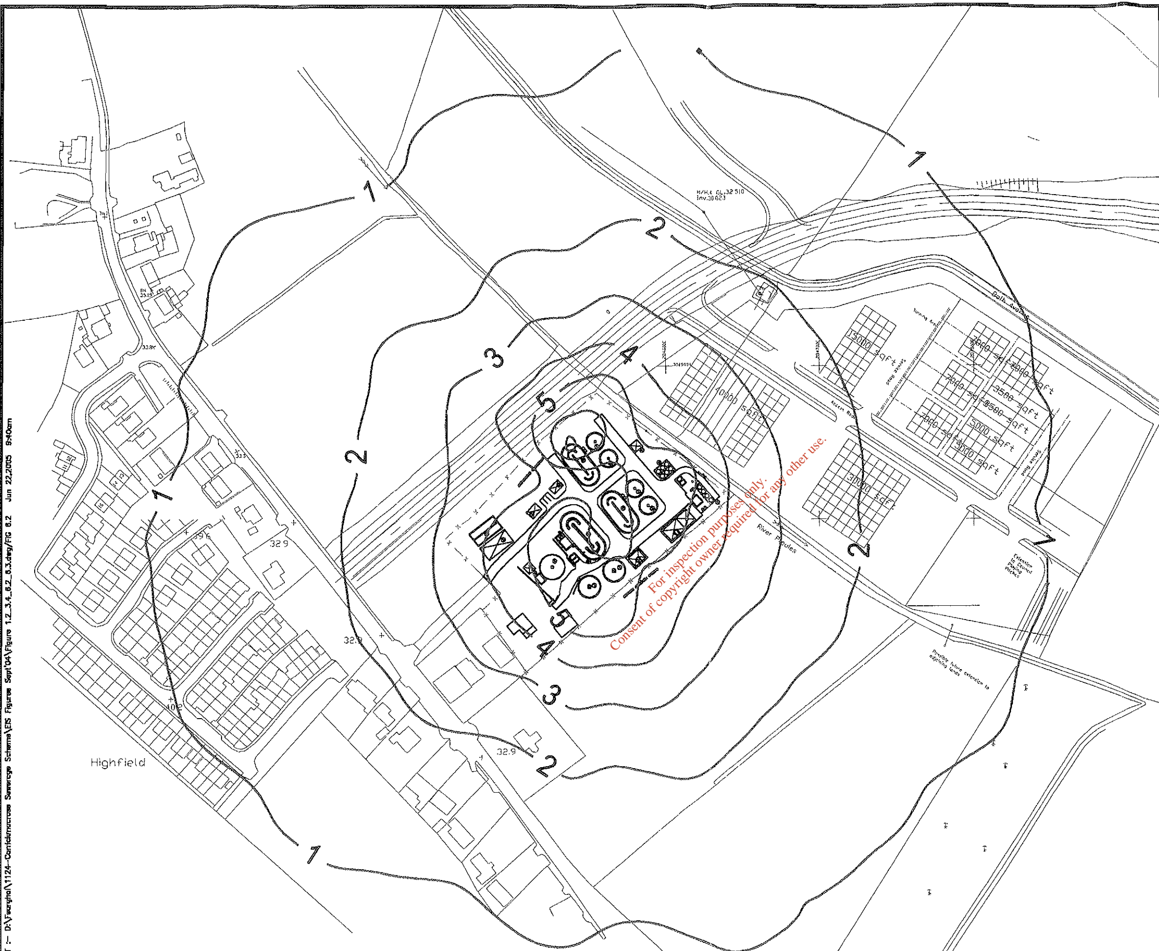
FIG 6.2: PREDICTED MAXIMUM 99.5 PERCENTILE OF SHORT-TERM ODOUR CONCENTRATIONS DUE TO EMISSIONS FROM PROPOSED EXPANSION OF WASTEWATER TREATMENT PLANT
