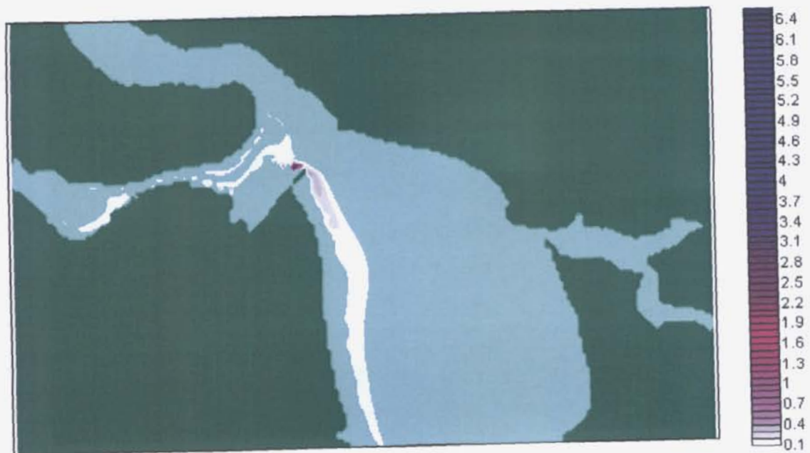
Figure A.8: Phosphate concentrations at low water on a spring tide ( \mu\text{g/l} )
