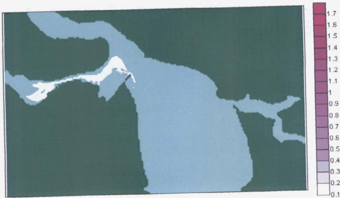
Figure A.7: Phosphate concentrations at mid ebb on a spring tide ( \mu\text{g/l} )
