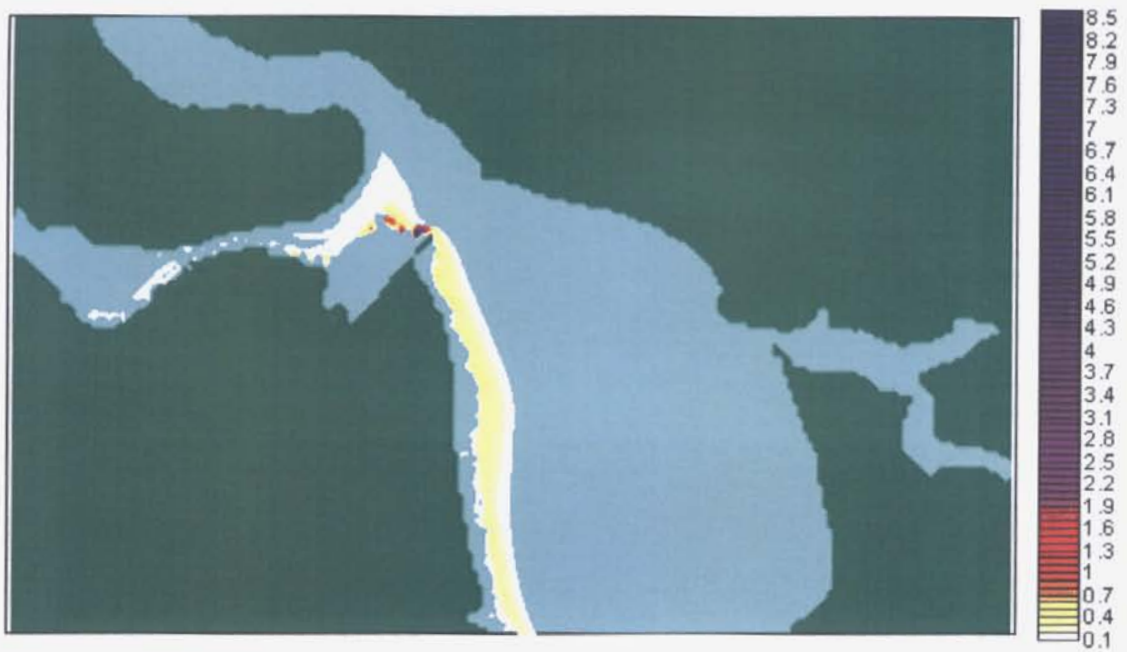
Figure A.28: VOC concentrations at low water on a neap tide ( \mu\text{g/l} )
