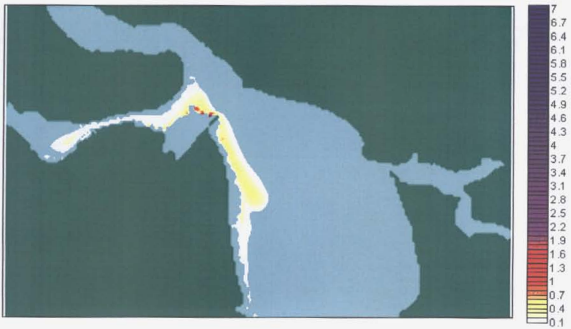
Figure A.27: VOC concentrations at mid ebb on a neap tide ( \mu\text{g/l} )
