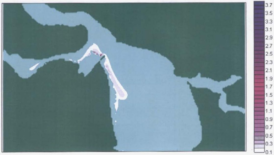
Figure A.3: Phosphate concentrations at mid ebb on a neap tide ( \mu\text{g/l} )
