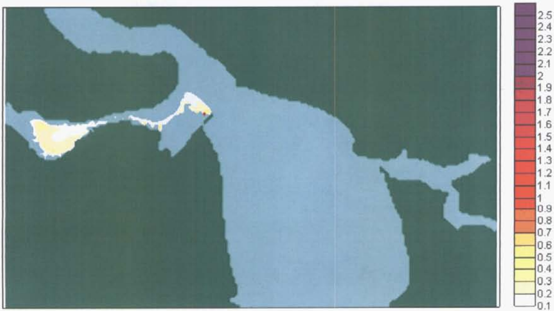
Figure A.30: VOC concentrations at high water on a spring tide ( \mu\text{g/l} )
