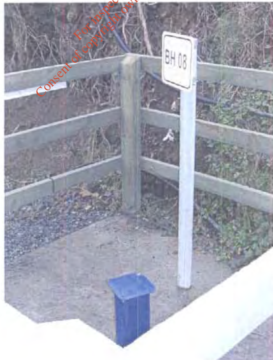
Plate 3.5.8: Groundwater Monitoring Borehole
