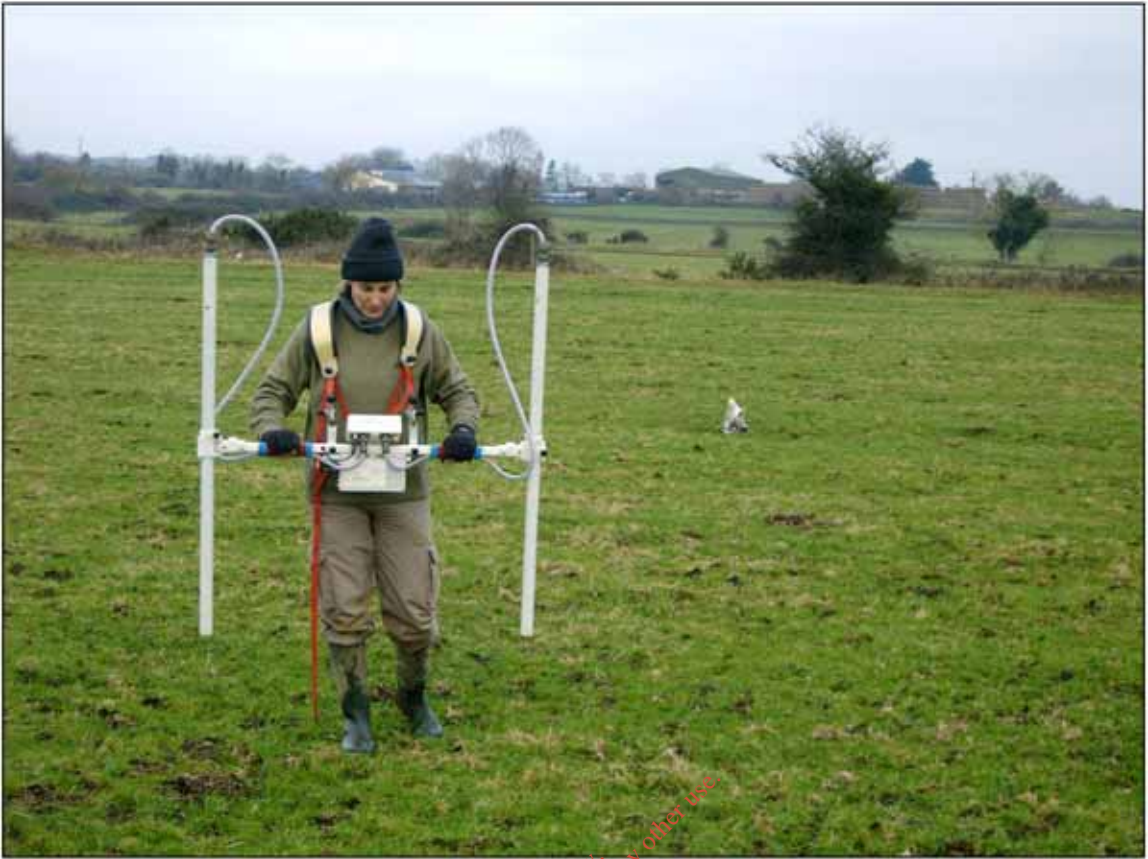
Plate 1 Field operative using the Barrington GRAD 601-2 dual sensor fluxate gradiometer
