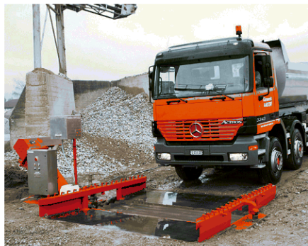
The approaching truck starts the wash cycle automatically via a photo sensor.
