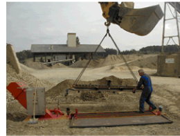
01:20 hours Fitting the wings and spray bars. Connecting the power and water
