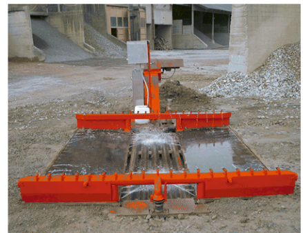
The wash water flows across the "wings" of the Dragon back into the recycling tank where it is treated ready for the next truck.
