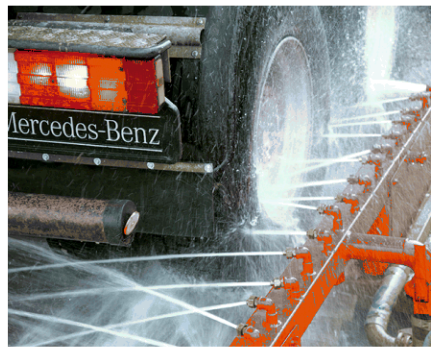
The wheels are washed intensively both from the sides and underneath as the truck drives slowly through.
