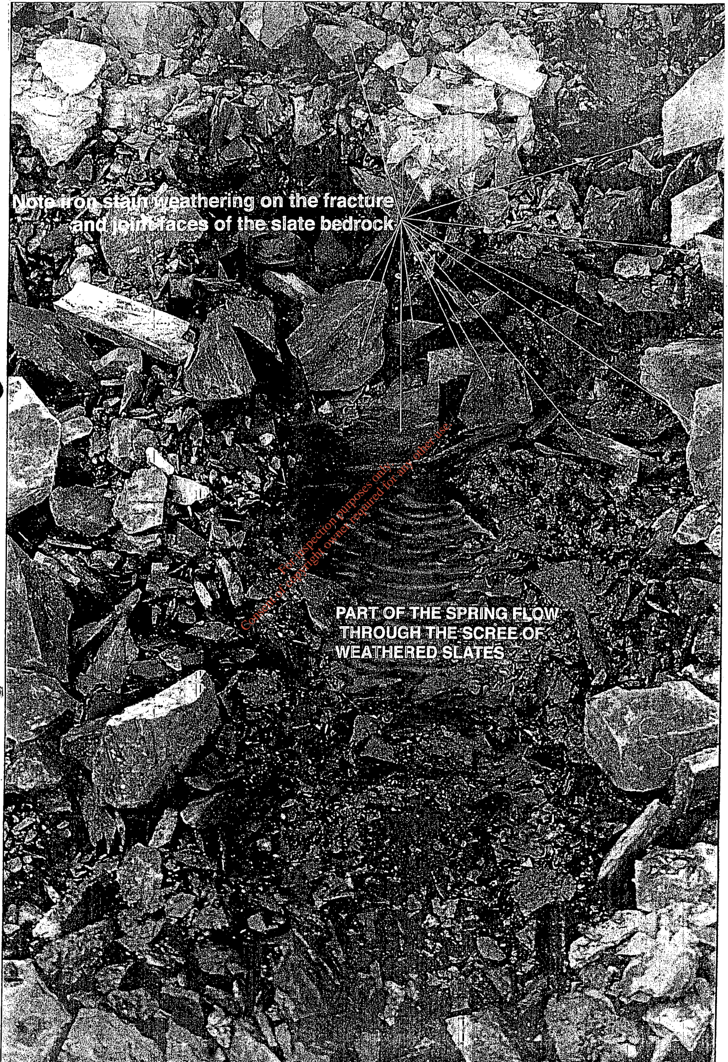
Figure 5 Part of the Spring seepage from the weathered and fractured Slate bedrock
