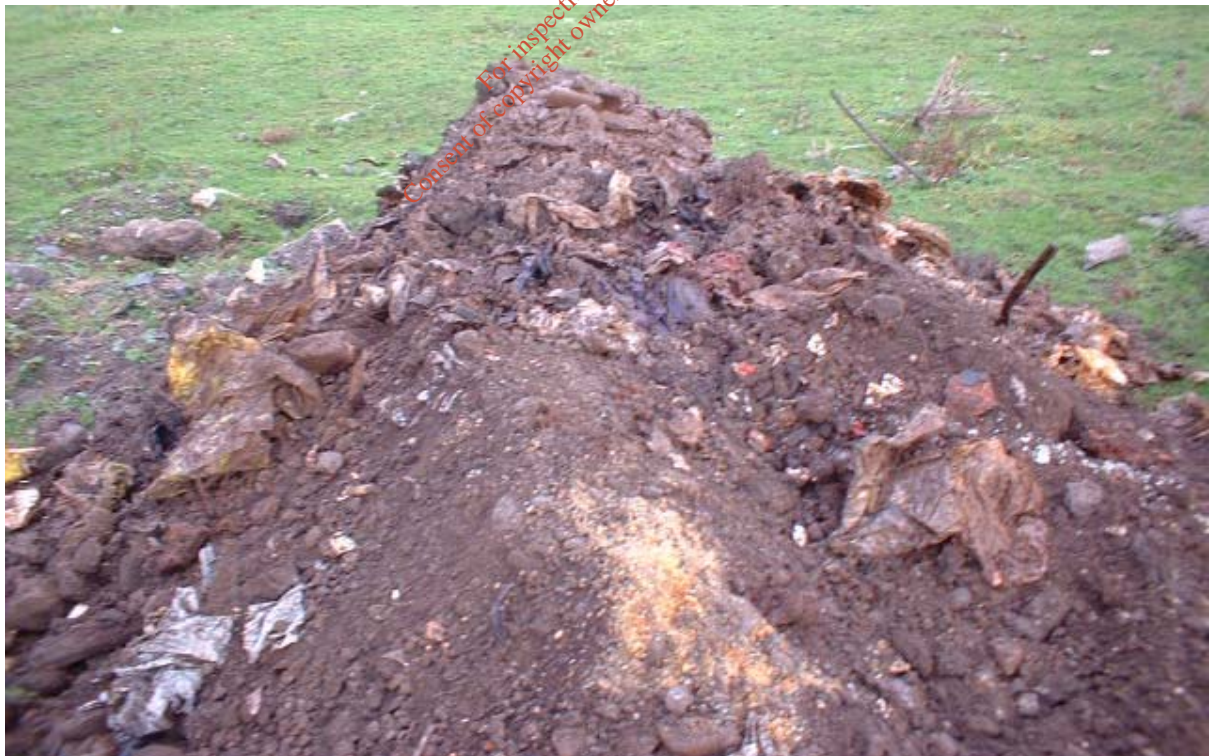
Plate 10 Trial Pit 5 Fill Material
