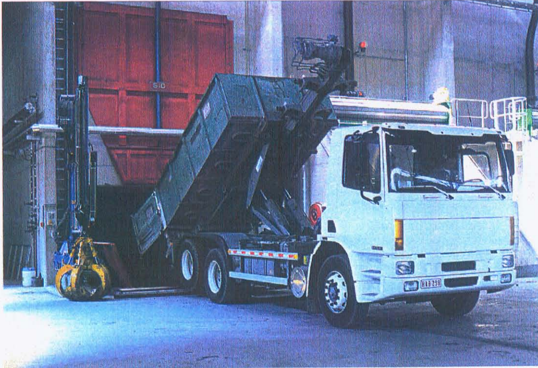
Truck unloading into Waste Bunker
