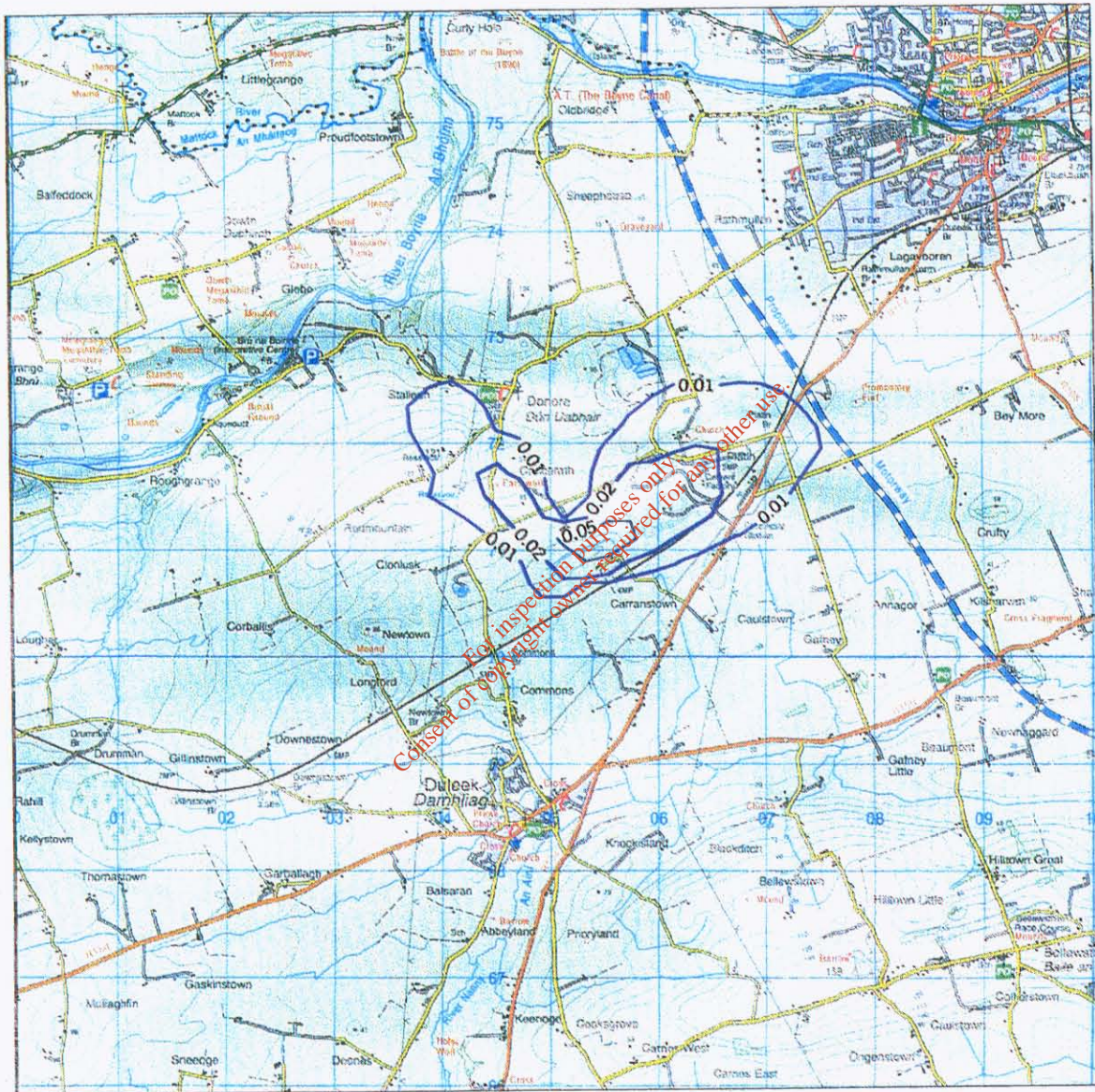
Figure 1.21: Predicted annual average Hg particle-bound deposition (mg/m 2 ) Maximum operation, Indaver Ireland Waste Management Facility
