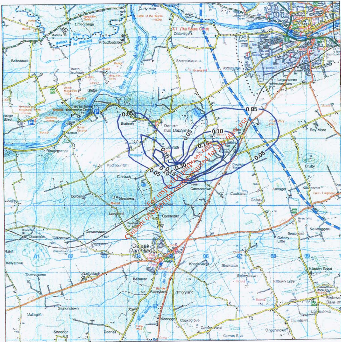
Figure 1.26: Predicted annual average arsenic total deposition flux (mg/m 2 ) Maximum operation, Indaver Ireland Waste Management Facility
