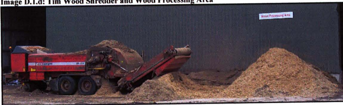
Image D.1.d: Tim Wood Shredder and Wood Processing Area
