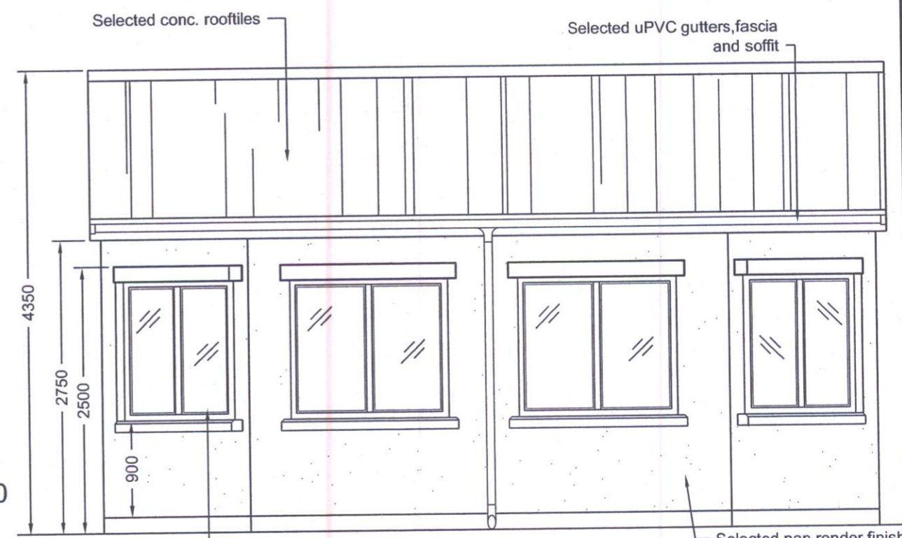
NORTH WEST FACING ELEVATION SCALE 1:50
