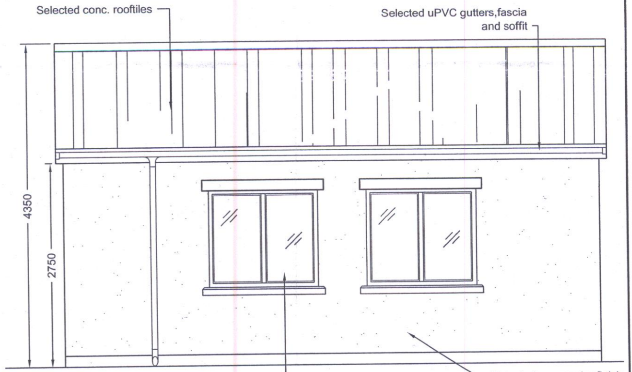
SOUTH EAST FACING ELEVATION SCALE 1:50
