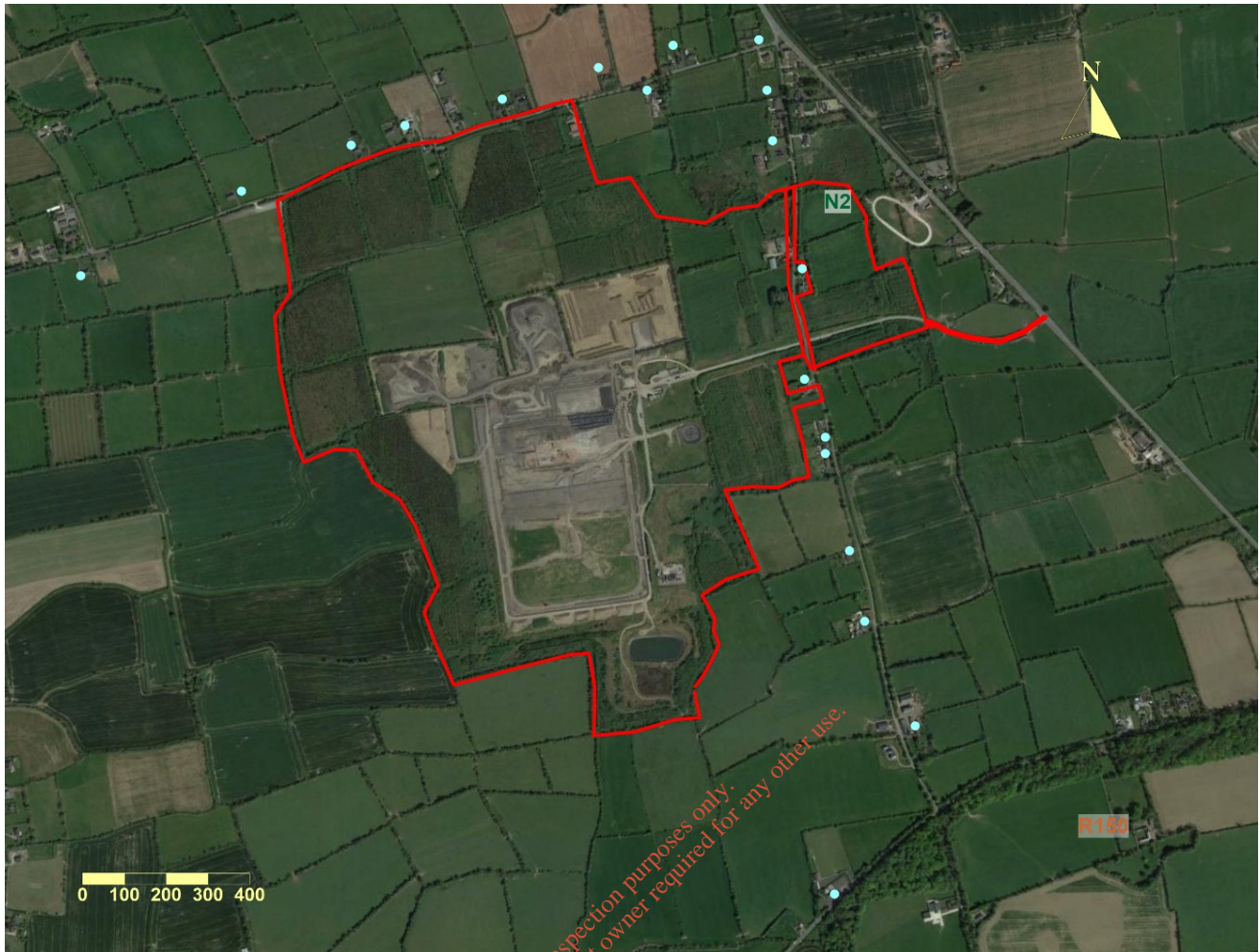
Figure 7-2: Location of sensitive receptors included within the dispersion model as blue dots with the planning boundary of Knockharley Landfill shown in red
