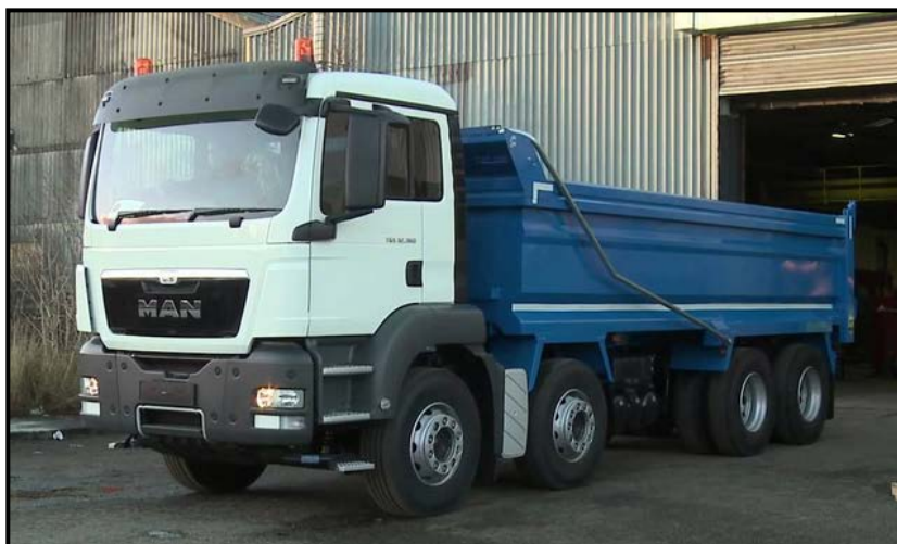
Plate 14.2.6 Example of an 8m Rigid Tipper Lorry typically used to transfer material
