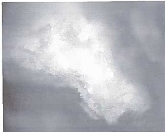
Fig. VII-5: \text{FeSO}_4 grain 300 \mu\text{m} in size consisting of cement with a passivating capsule of reaction products and the intact core of reactive \text{FeSO}_4 \cdot 7\text{H}_2\text{O}
