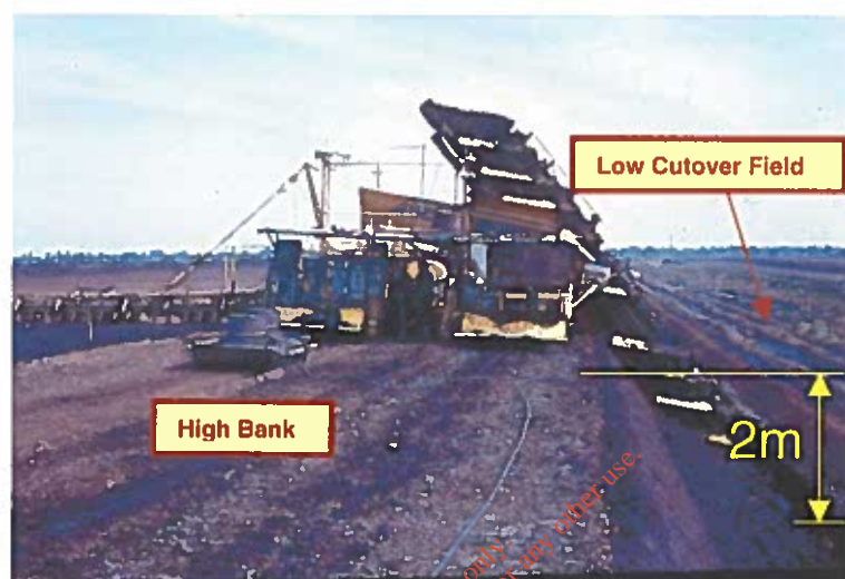
Figure 11 Machinery Cutting Sod Peat on High Peat Bank
