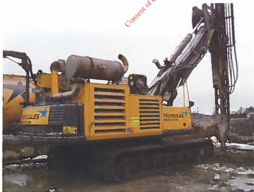
Figure 6 Column Stabilisation Rig in Operation
