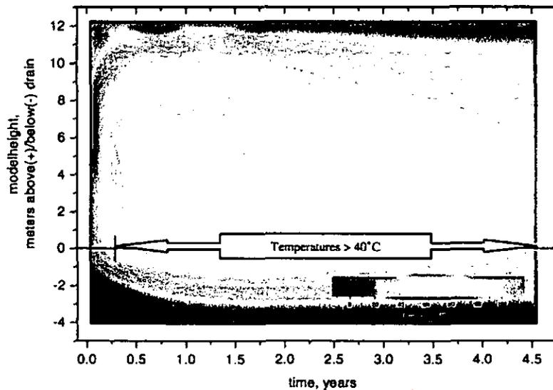
Fig. 9. Predicted temperature development in simulation no. B. Initial heating rate for the 3–6 weeks stored bottom ash was set to  $25 \text{ W m}^{-3}$ , final bottom ash height to 10 m (deposited in 3 weeks to its final height). Surface sealing was installed directly after the deposition of the bottom ash.
